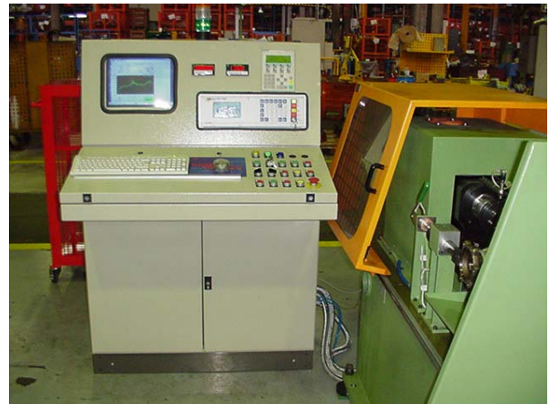
- Example of installed quality control system (gearboxes) -
